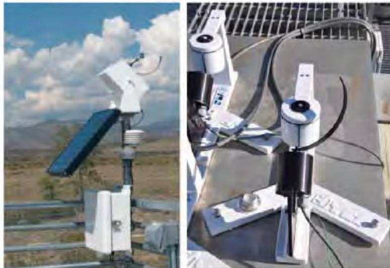
**Figure 3-12. Two commercially available RSRs: Irradiance, Inc. Model RSR (left) and Yankee Environmental Systems, Inc. Model SDR-1 (two units shown on right)**
