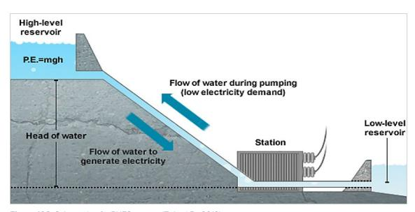
Figure 106: Schematic of a PHES system (Zohuri B., 2019)
