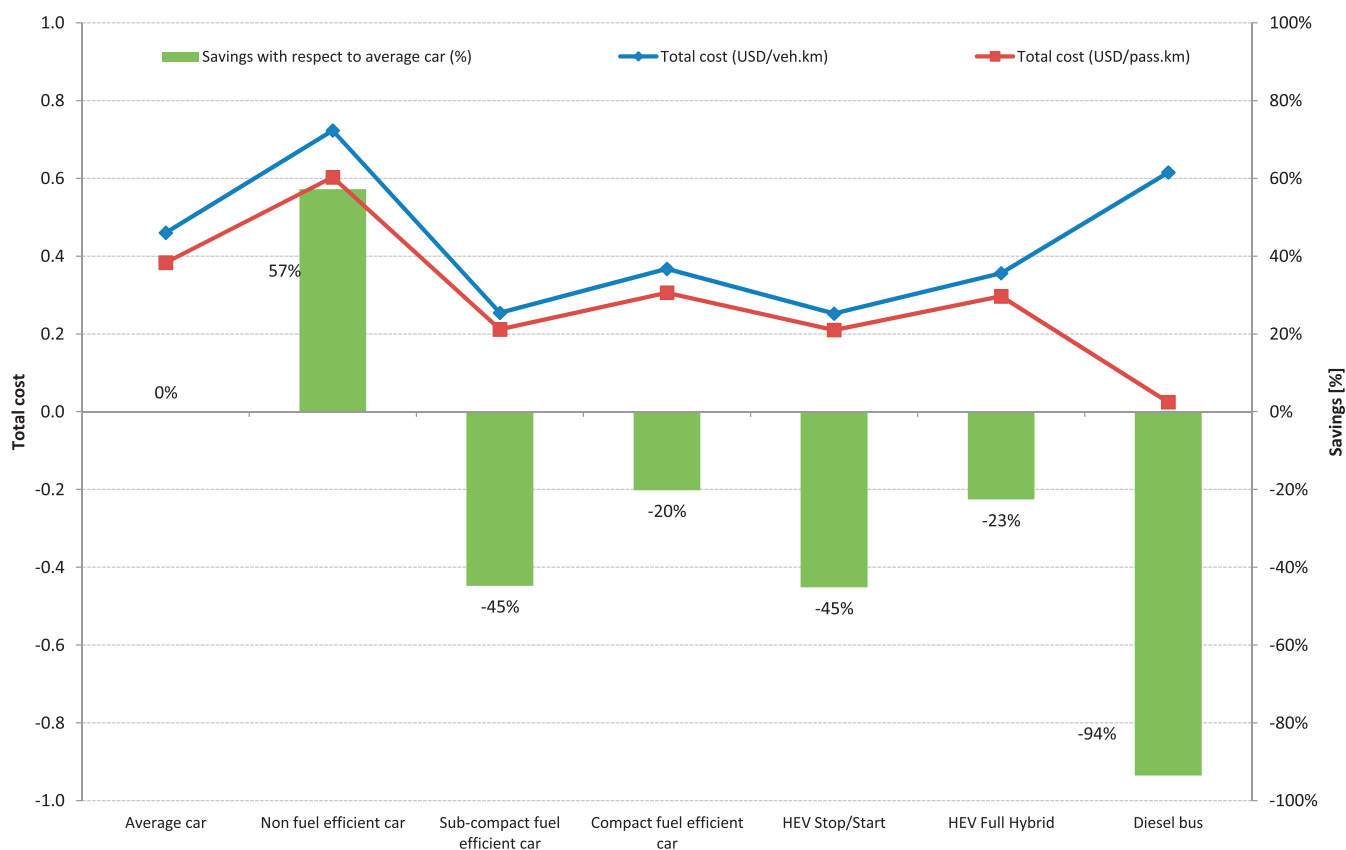
Fig. 36 - Total vehicle costs of the studied transport technologies under GBA peak driving conditions.
