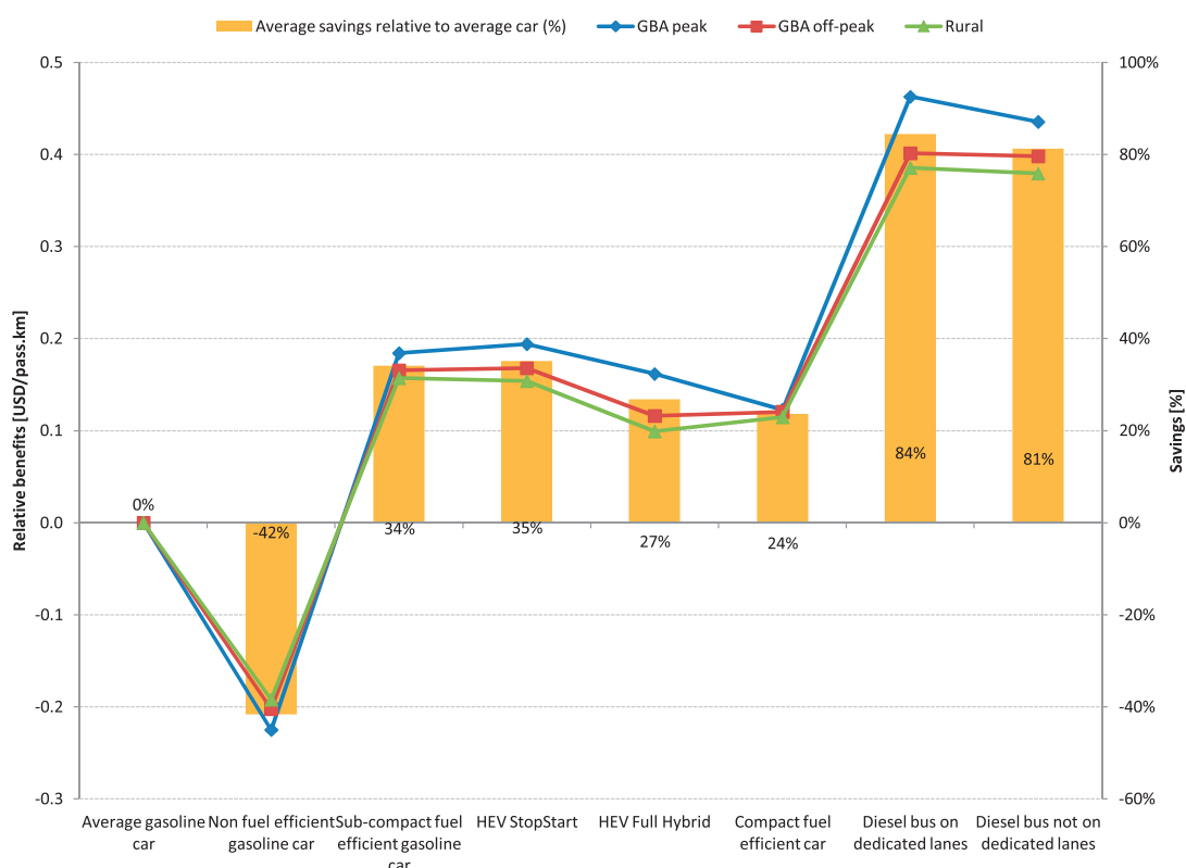
Fig. 37 - Car users benefits of transport technologies relative to average car under GBA driving conditions.
