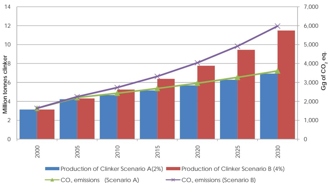
Figure 3-7 Projected clinker production and CO<sub>2</sub> emissions under scenario A and scenario B
